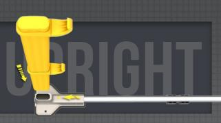
Put handrail and kneerail onto tube fixing then fix them by tightening screw
